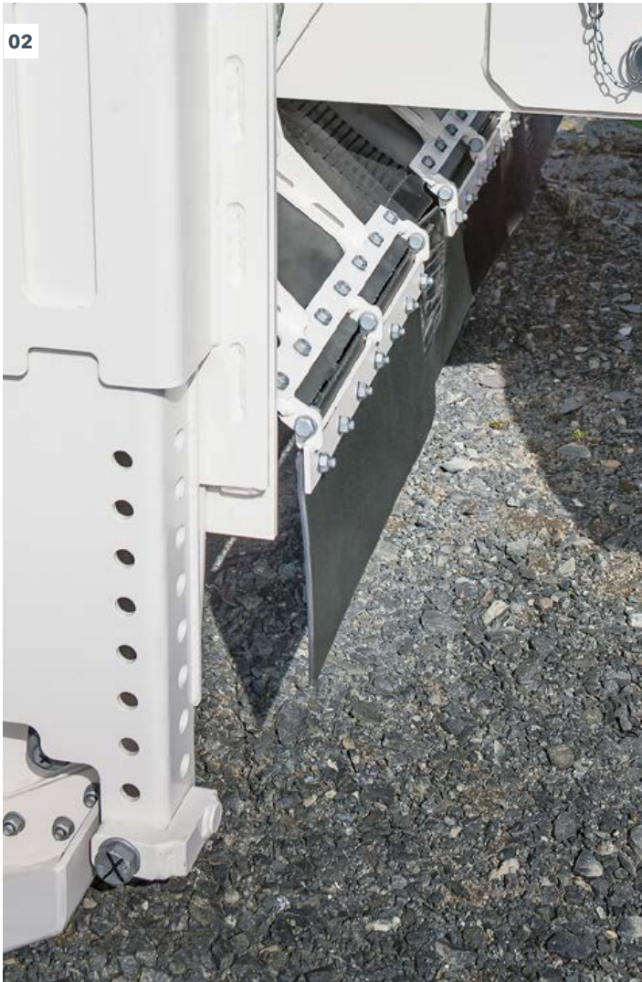
01 The stone guard is proving its worth in operation: no flying stones and less dust.
