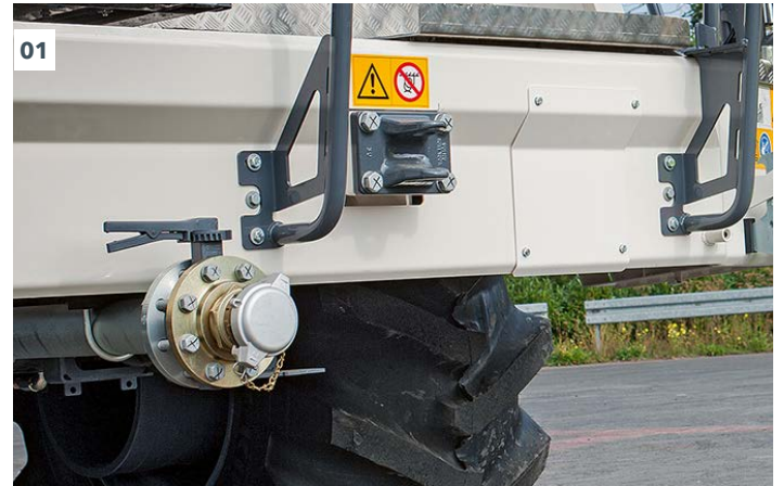
01 All of the hose connections are attached to the front cross member.
