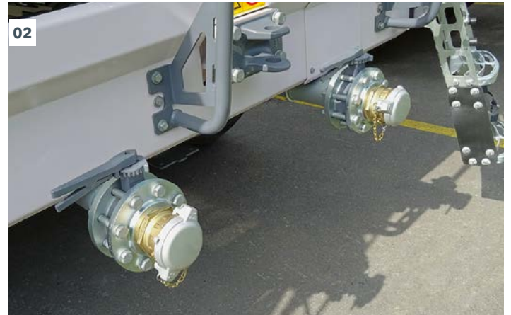
02 Connections for water and emulsion are easily accessible.
