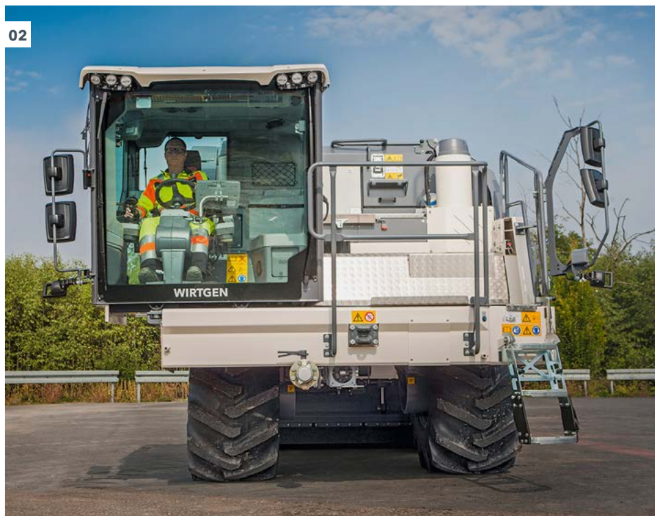
01 - 02 The operator's cabin can be moved far to the right hydraulically, allowing the operator to look past a recycling train traveling ahead.
