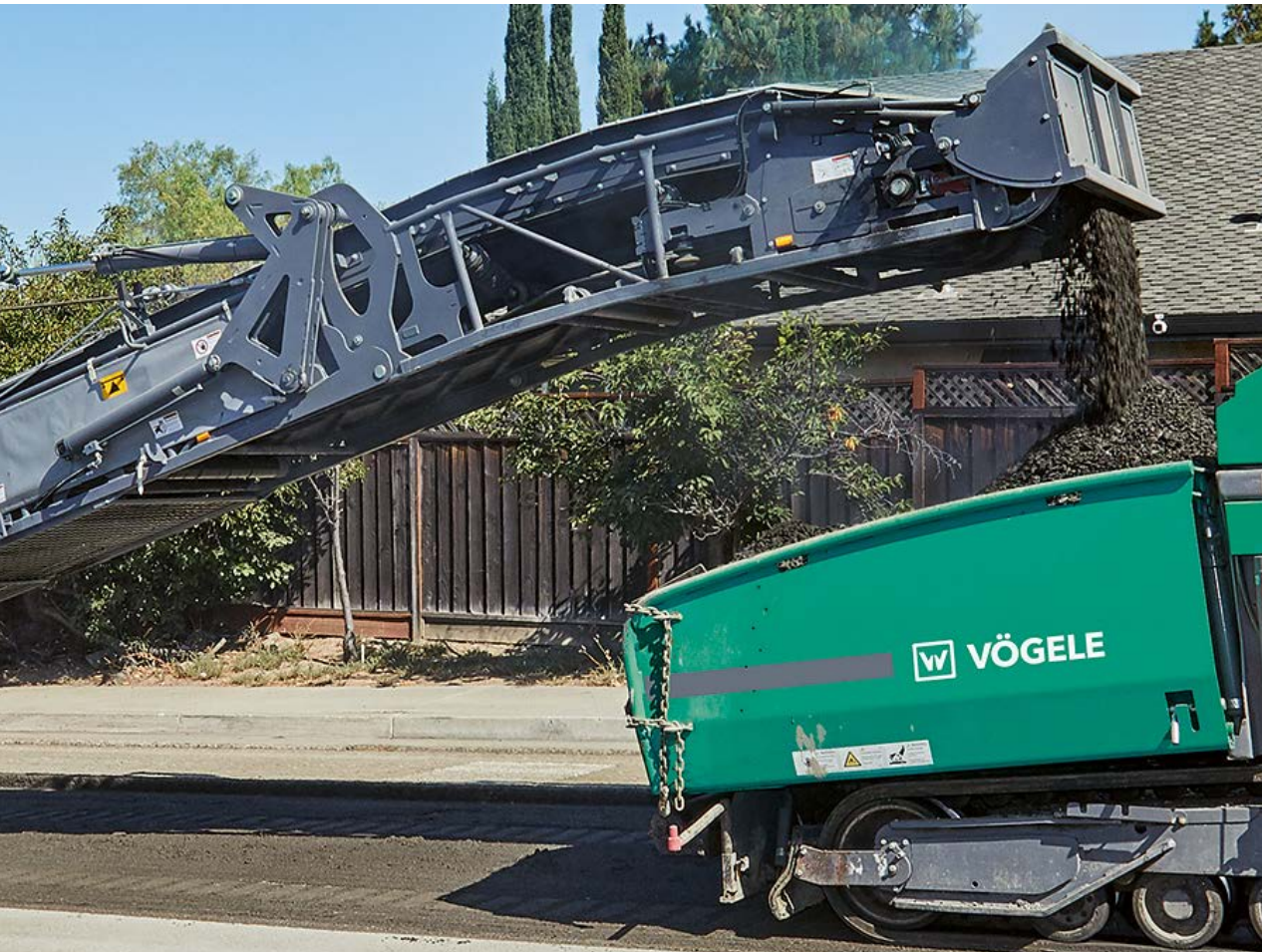
01 The W 380 CR(i) recycles road pavements at a mixing capacity of up to 800 t/h.
