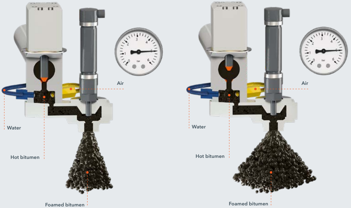
Foamed bitumen is produced by injecting compressed air and water into hot bitumen in a controlled process.
