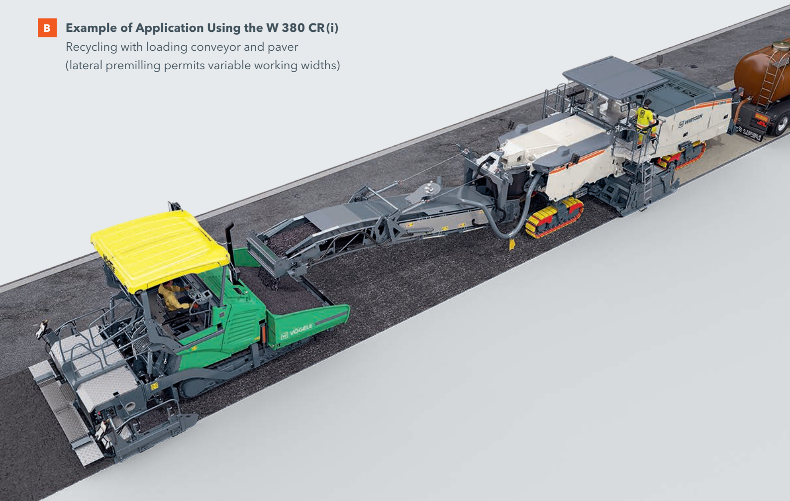
01 The W 380 CR(i) recycles road pavements at a mixing capacity of up to 800 t/h.
