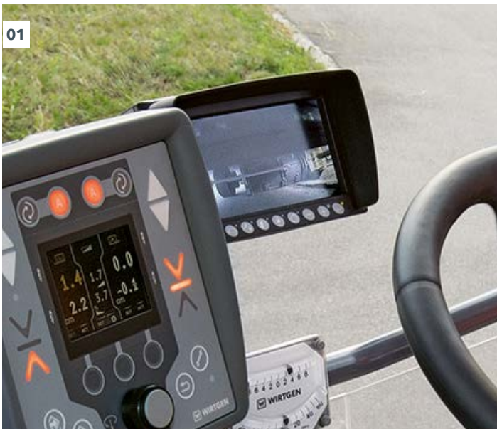
01 The camera's ability to see and display key work areas enhances performance and quality. 02 The operator always has an unobstructed view of the right side plate.
