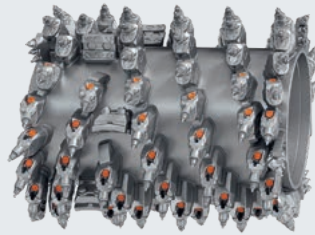
Standard Milling Drum Milling width: 1,200 mm Milling depth: 0 - 330 mm Tool spacing: 15 mm
