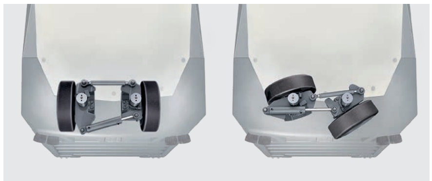
The front axle enables large steering angles.
