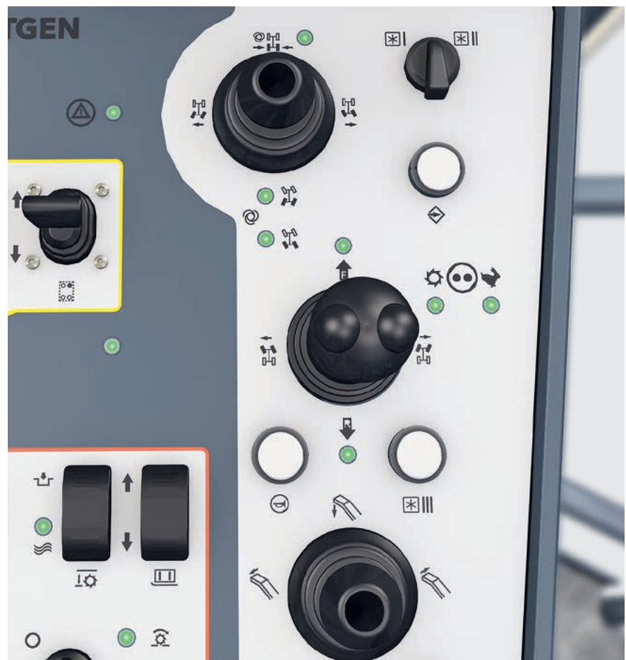
Clearly structured control panel with language-neutral labelling.
