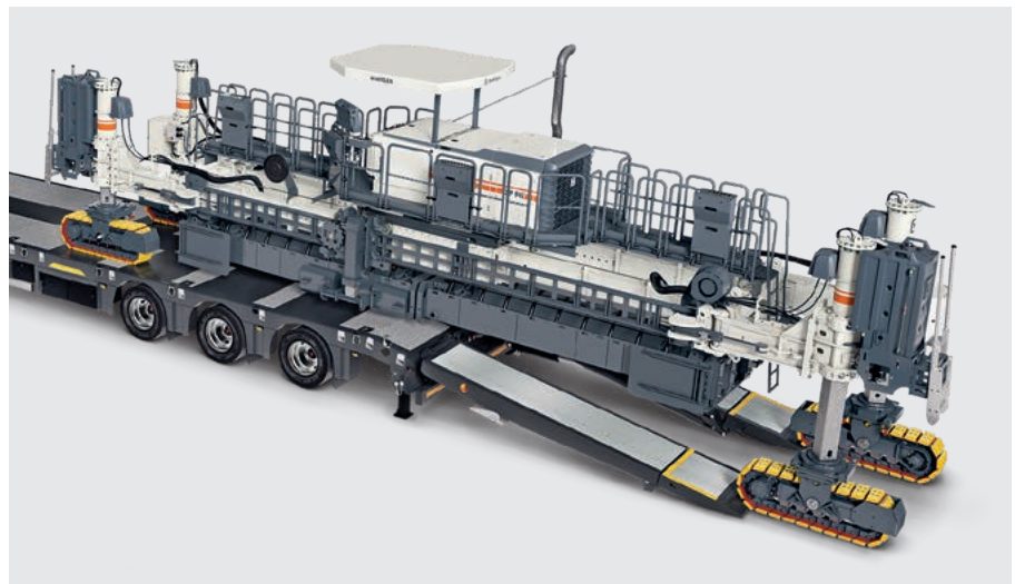
Hydraulic swivel arms for easy transport and a high degree of flexibility on the job site.
