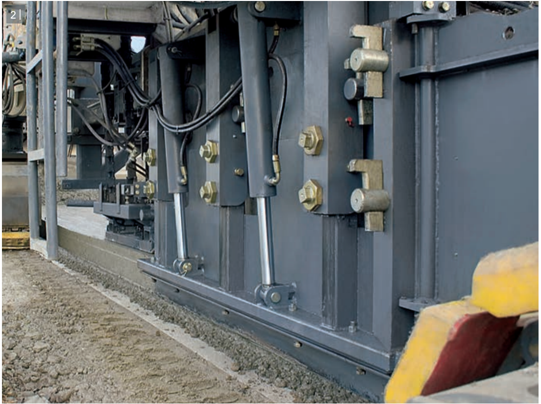
2 | Hydraulically adjustable side-plates ensure clean concrete edges.
