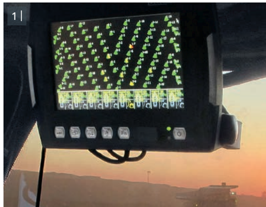
1 | Worn picks are identified by means of an optical measuring process and then marked in color on a screen.
