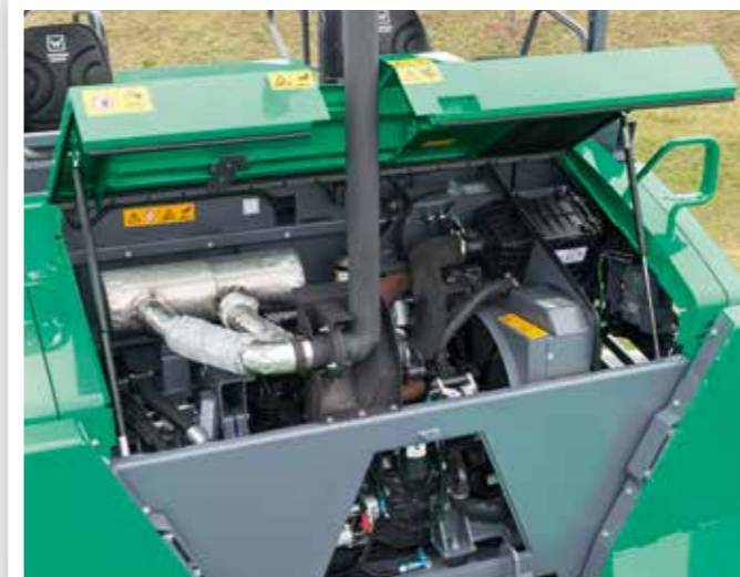
The large cooler assembly is made up of three parts. It ensures that engine coolant, charge air and hydraulic oil are maintained at the optimum temperature.
