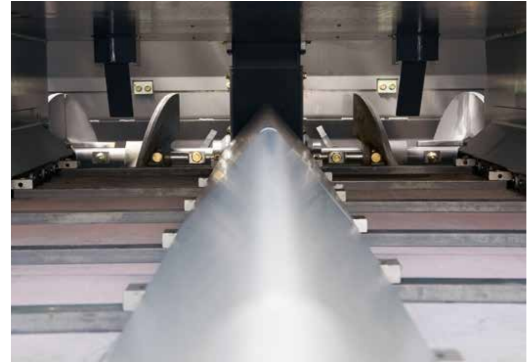
The conveyor can be reversed at the touch of a button. Return transport of the mix is stopped automatically. The conveyor can be switched to the no-load function just as quickly.
