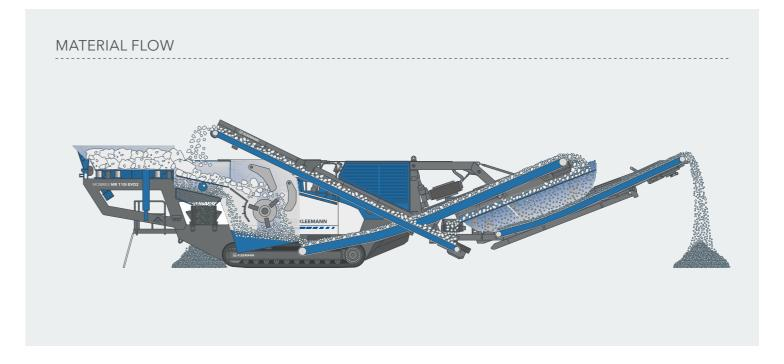
The MOBIREX MR 110(i) EVO2 stands out with its optimal material flow concept: The system widths are extended over the entire plant in the direction of material flow. This means that the material flow is not restricted and material bridging can be effectively avoided. The Continuous Feed System makes the operator's work easier,
