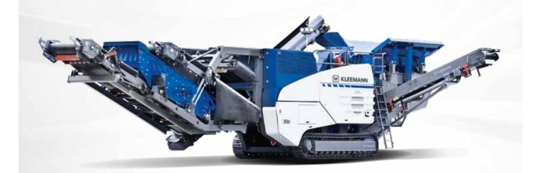
**Track-mounted impact crusher** Used in natural stone and recycling
