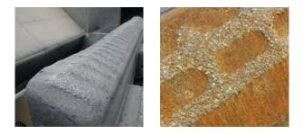
> Different arrangement of the ceramic inserts in the basic material
