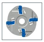
Wear due to replacing the blow bars too late
