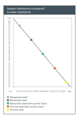
An increase in the steel's wear resistance (hardness) is usually accompanied by a reduction in toughness (impact resistance) of the material.
